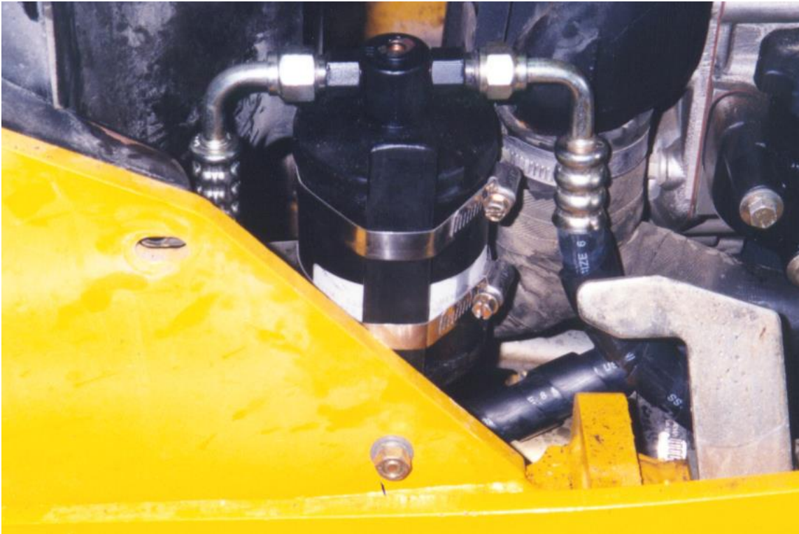
Drier in place on right side frame member. Nut showing is for mounting bracket.
